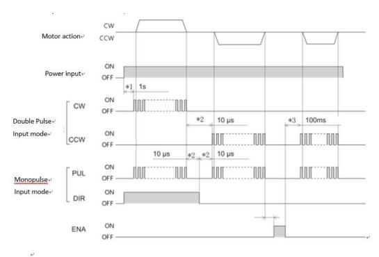
\* 1 driver is powered on and motor parameters are identified. Please send pulse instructions after 1S.
