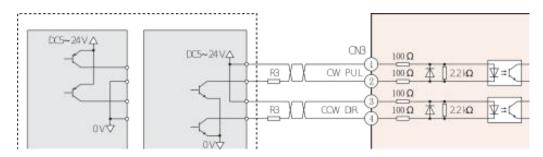
When the pulse input is an open collector, the wiring is as follows:
